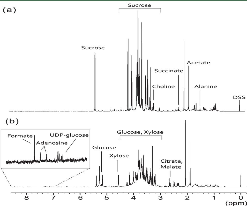
**Figure 5.** Representative 600 MHz  $^1\text{H}$  nuclear magnetic resonance (NMR) spectra of ginsengs: China (a) and Korea (b).
